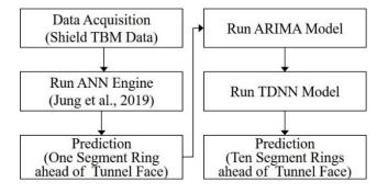
Fig. 1 Conceptual diagram of steps for predicting ground conditions
